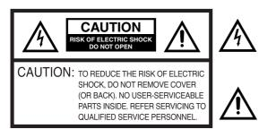
The lightning flash with arrowhead symbol, within an equilateral triangle is intended to alert the user to the presence of uninsulated dangerous voltage within the product's enclosure that may be of sufficient magnitude to constitute a risk of electric shock to persons.
